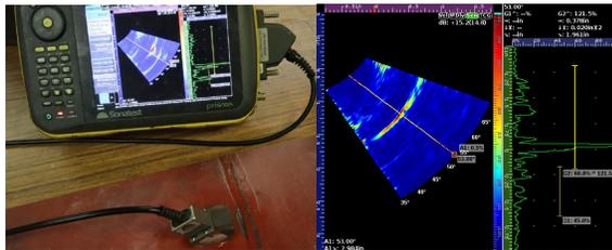
Figure 2. PAUT inspection and result for one of the butt weld MG plates
