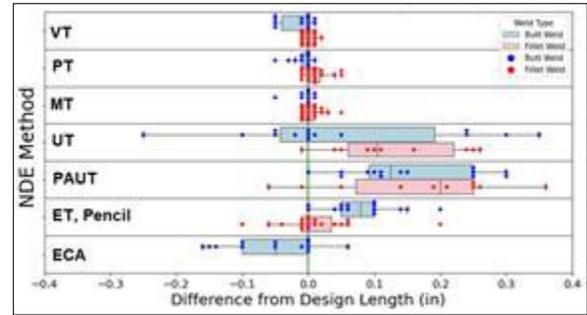
Figure 4. Boxplots showing sizing differences for each NDE methods in butt weld and fillet weld MG plates
