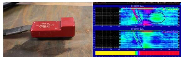
Figure 5. Eddy current array (ECA) inspection result for one corrosion plate
