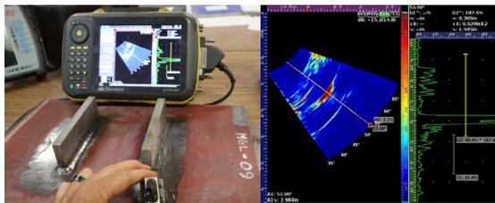
Figure 3. PAUT inspection and result for one of the fillet weld MG plates
