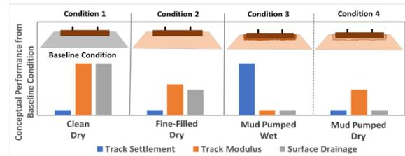
Figure 2. Conceptual performance of four ballast conditions
