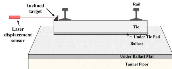
Figure 2. Configuration of a laser displacement sensor
