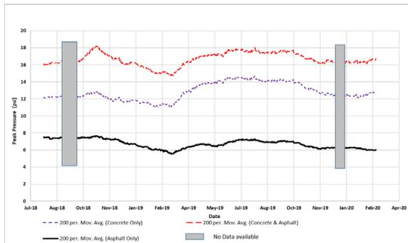
Figure 3. Moving average of peak pressure measured over time in the portal transition area
