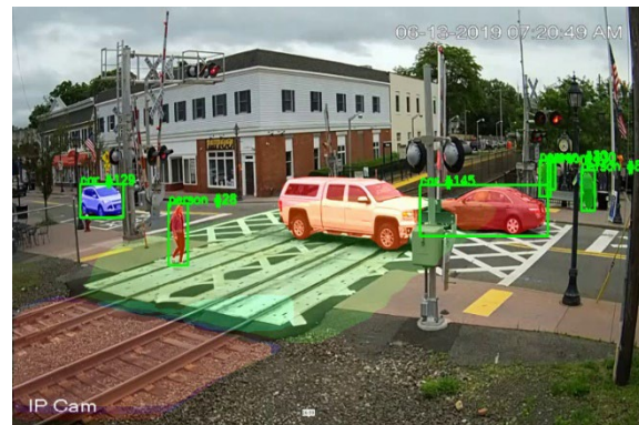
Figure 1. Example of Video Processing Output Showing Pedestrian and Vehicles Traversing a Grade Crossing in Ramsey, NJ
