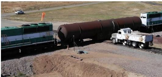
This test used cryogenic liquid nitrogen (LN2) as a stand-in for the cryogenic materials used as a
