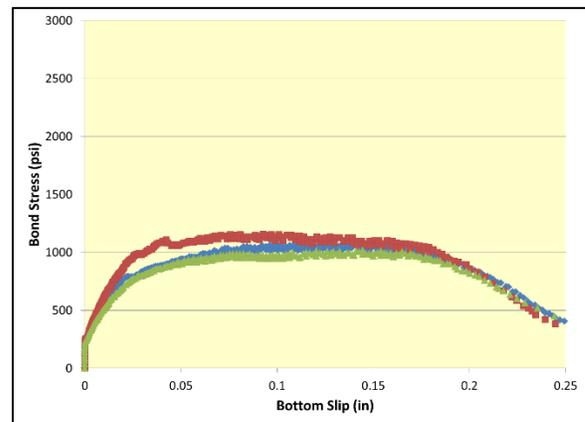
Figure 9: Bond-versus-slip curves for wires with dot-patterned indents
