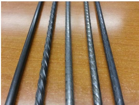
Figure 2: Five different 5.32-mm-diameter wires with different indentation types were utilized
