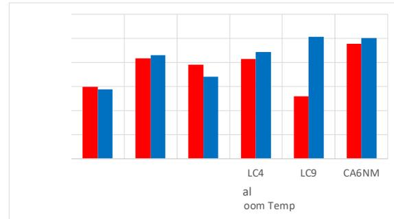
**Figure 3. Yield strength at -60 °F and at room temperature for the six steels**
