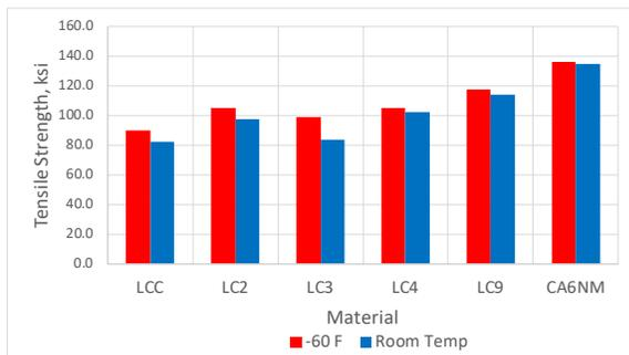
**Figure 2. Ultimate tensile strength at -60 °F and at room temperature for the six steels**
